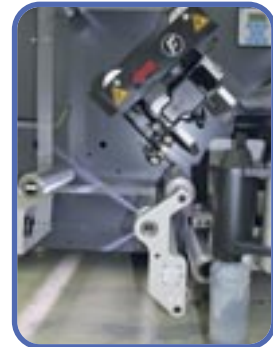
fleyeVision OCR, camera inspection of the back side numbering
