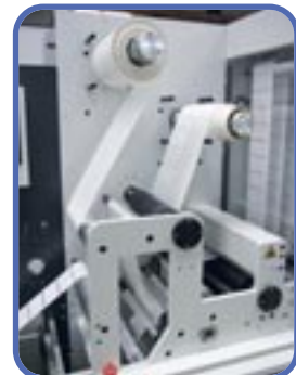
Leader and trailer (fully automatic label dispensing for leader and tails)
