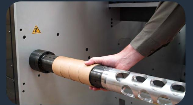
A product of the ABG Connect automation portfolio, ABG's core cutting solution allows you to produce made to measure cores on demand for each new job.
